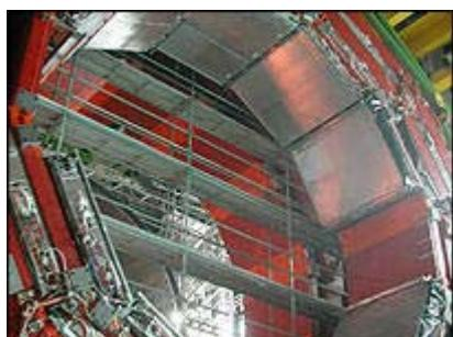
The CMS is constructed from different layers in an "onion" structure
